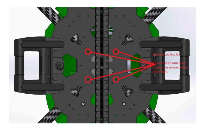
**Payload Mount Rail:** are a key function on mounting external payloads to the aircraft, it is a simple Picatinny rail that when coupled with the quick disconnect make it easy to attach and move payload articles. Make sure the rail is securely fastened and that the quick release is correctly attached. If you feel play in either the quick release of the mounting of the rail, inspect and adjust as necessary.
